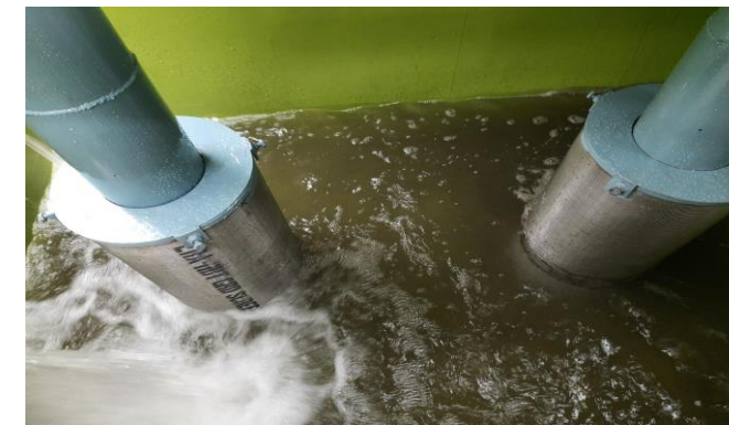
GRD filter inside filtration Cassette
