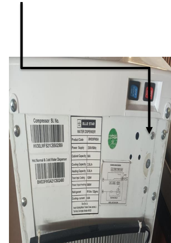
Cooled water temperature control ( 6 deg to 16 deg)
