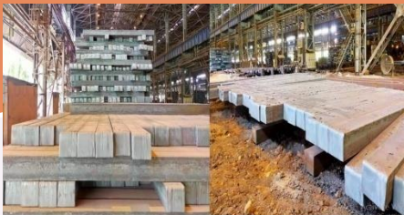
Blooms Stacked in Zig-Zag Pattern due Non-Functioning of Dropping arrestors
