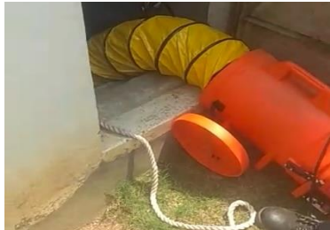
Air blower for confined space
