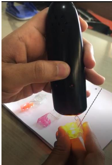
Infra Red Sensor DEVELOPED to check authenticity of seals by verifying the transparency
