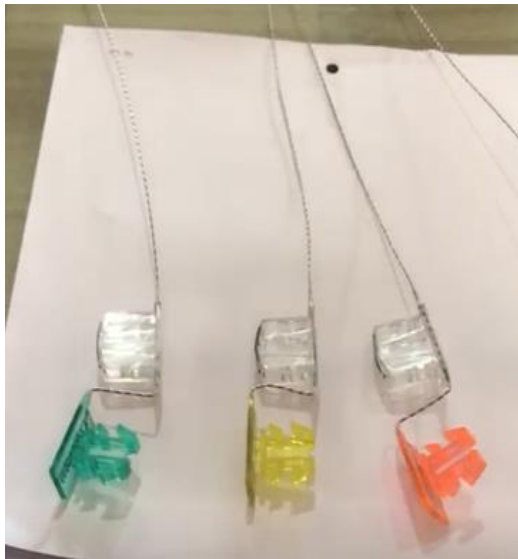
New Polycarbonate seals of pre-determined transparency by doping of a unique agent
